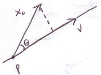
$\frac{\|(x_0-p) \times v\|}{\|v\|} = \text{distance from } x_0 \text{ to line } l(t),$
